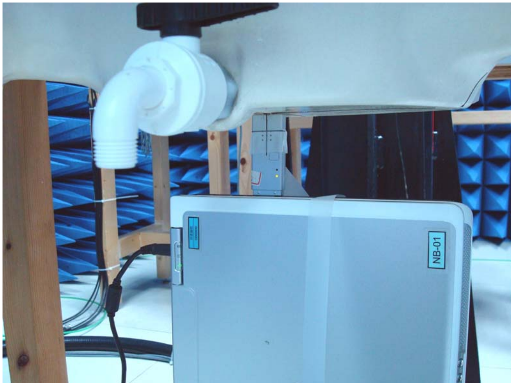
Figure 14. Body SAR Test Setup (Flat Section)_Bottom
