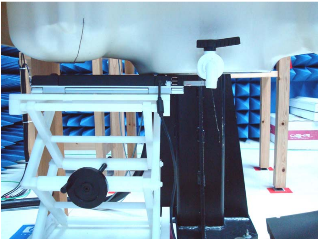
Figure 12.Body SAR Test Setup (Flat Section)_Tip
