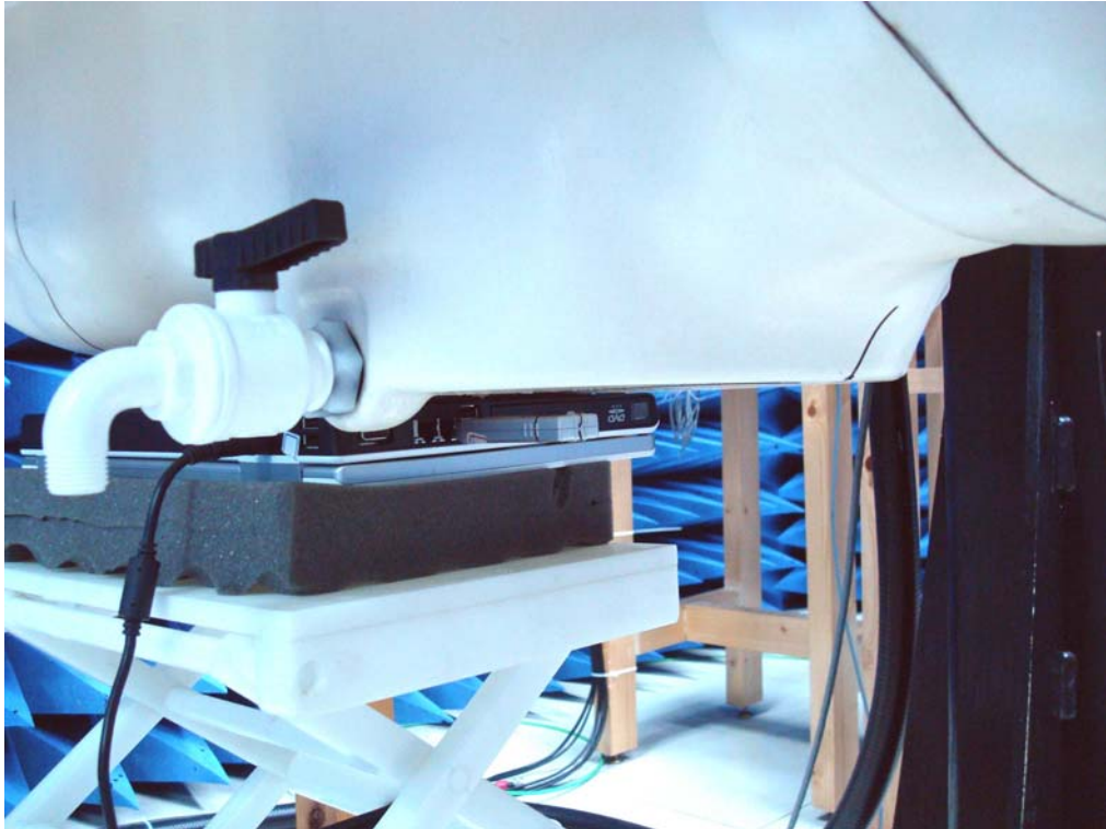
Figure 11.Body SAR Test Setup (Flat Section)_Tip
