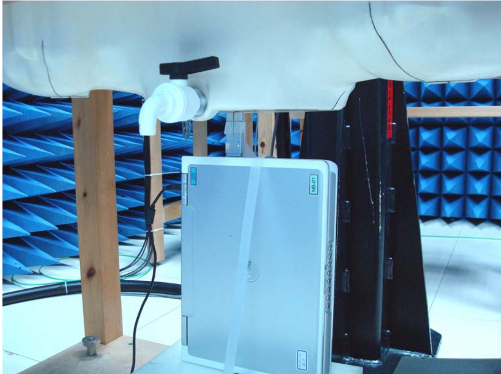
Figure 13. Body SAR Test Setup (Flat Section)_Bottom
