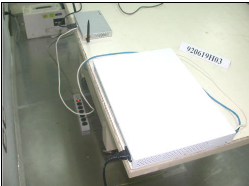
RADIATED EMISSION TEST (With Adapter)
