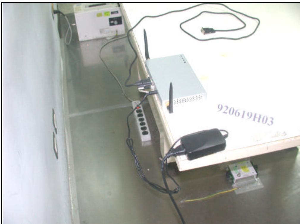
**CONDUCTED EMISSION TEST (With POE)**
