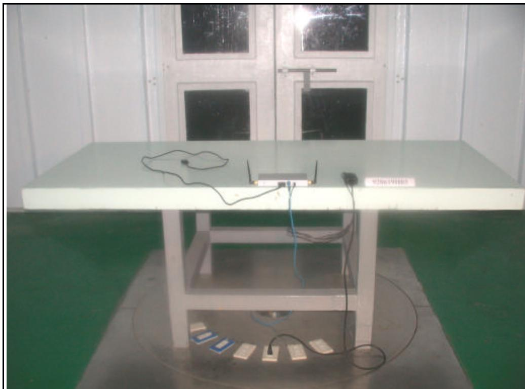
RADIATED EMISSION TEST (With POE)
