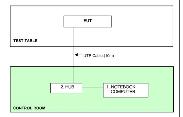
**NOTE:** 1. Support units 1&2 were kept in the control room during the test.
