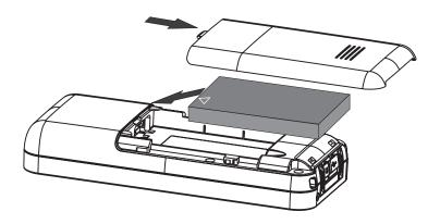
**3.** Replace Battery Compartment Cover — Slide the battery compartment cover back onto the phone until it clicks firmly into place.
