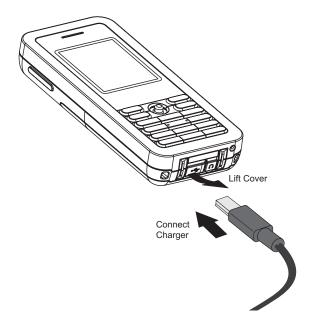
Disconnect the Power Charger — When the battery is fully charged, remove the power charger from the phone and push down the charger port's rubber cover.
