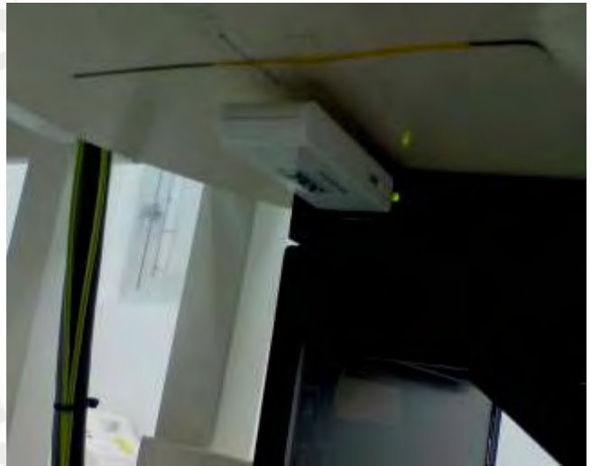
Fig.3 Back side of the EUT is paralleled with flat phantom, and spacing between EUT and Phantom is 4 mm.
