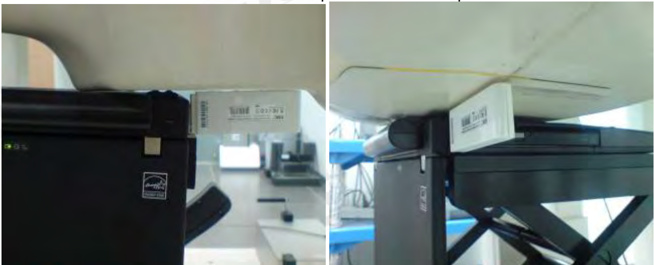
Fig.6 Bottom side of the Notebook is paralleled and contacted with flat phantom, and right side of the EUT is paralleled with flat phantom.
