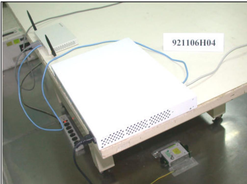
RADIATED EMISSION TEST (With Adapter)
