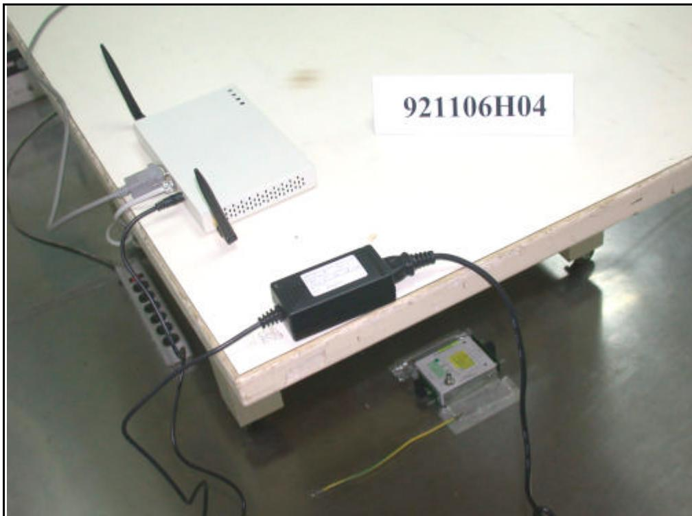
**CONDUCTED EMISSION TEST (With POE)**
