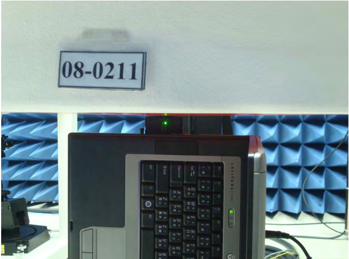
Figure 11. Body SAR Test Setup (Flat Section)
