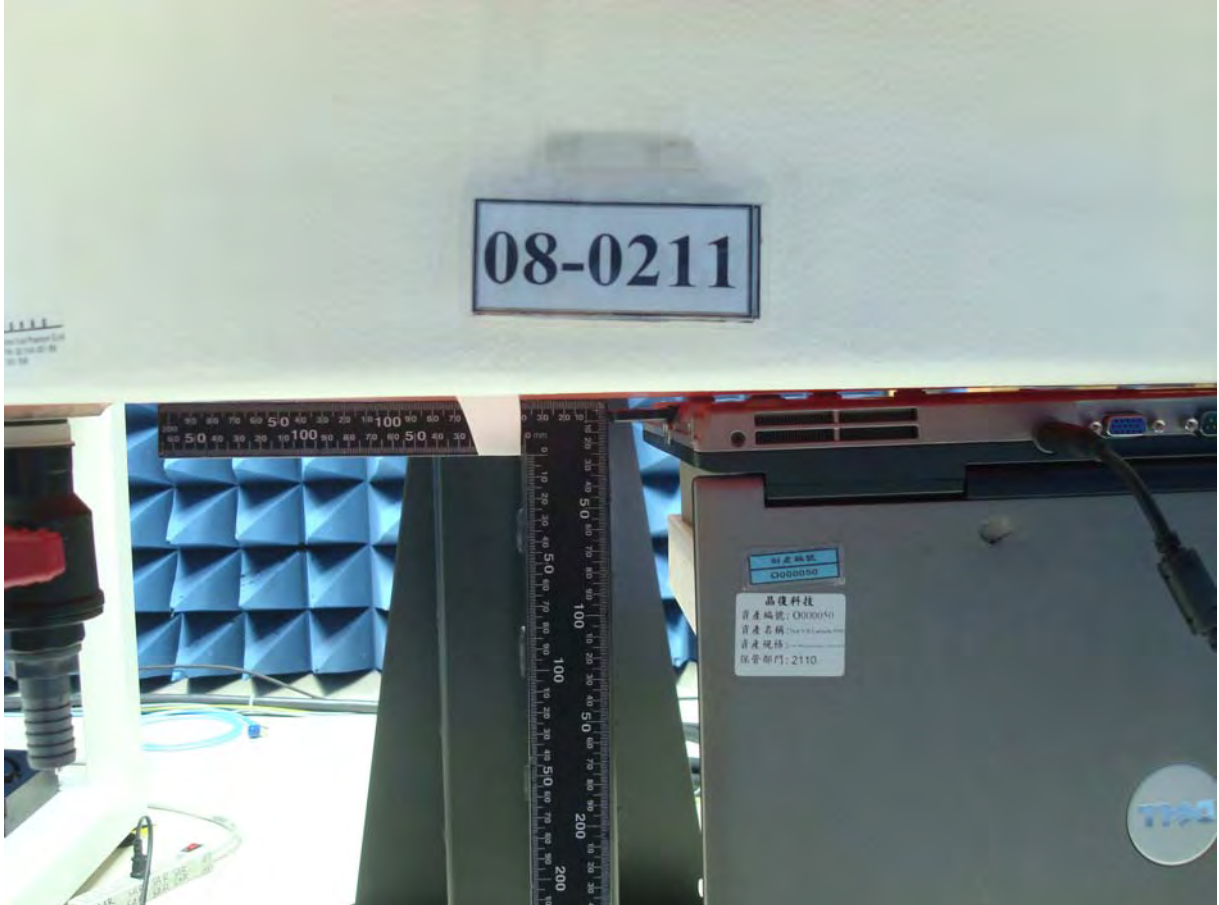
Figure 12. Body SAR Test Setup (Flat Section)
