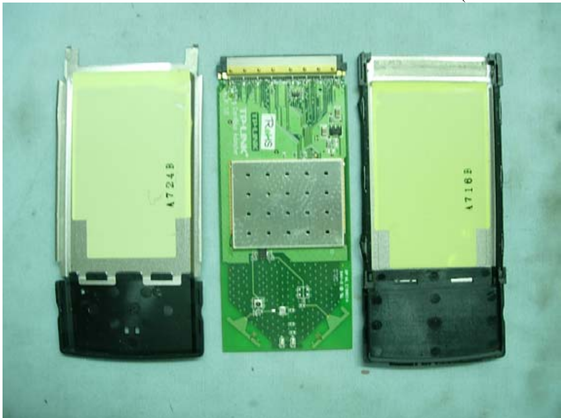
Figure 4 Internal View (Removed Covers)
