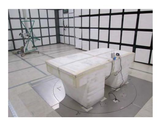
Test Configuration: Above 1GHz / Test Mode: Mode 1
