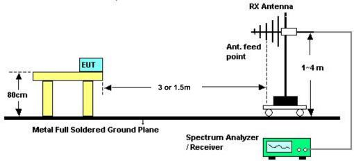
Above 10 GHz shall be extrapolated to the specified distance using an extrapolation factor of 20 dB/decade form 3m to 1.5m.
