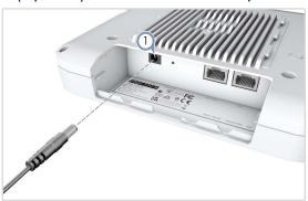
When not connected to a PoE source, connect the AC power adapter to the DC power jack on the AP and then plug the adapter into a nearby AC power source.
