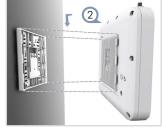
At the installation location on the wall, use the mounting bracket to mark four holes for the wall plugs and screws (included in the screw kit)
