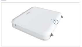
When operating normally, the System LED should be on green.
