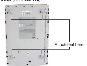
Position the BSG on a desktop. Make sure you leave enough space around the unit for ventilation and access to the cables. Install the power supply next to the BSG. The power supply must be within 1.5 m (5 ft) of the BSG and within 1.5 m (5 ft) of the AC power outlet (wall outlet or universal power supply).
