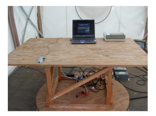
Radiated Emission Test Setup - Rear View
