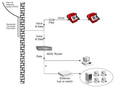
Figure 2-2. Installing without a Splitter
