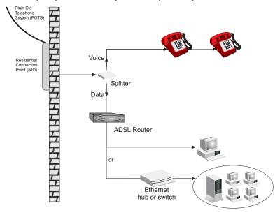
Figure 2-1. Installing with a Splitter
