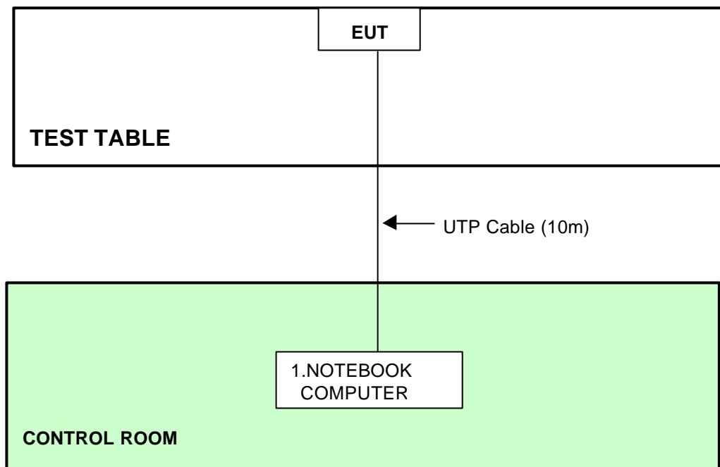
**NOTE:** 1. Support unit 1 was kept in the control room during the test.
