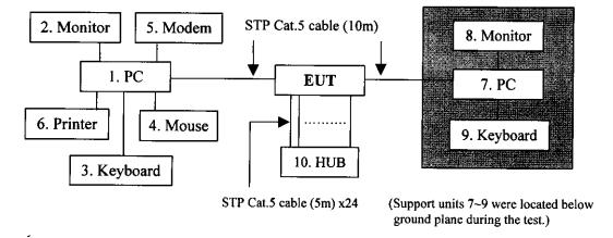
Both conducted and radiated testing were performed according to the procedures in ANSI C63.4: 1992. Radiated testing was performed at an antenna to EUT distance of 10 m on an open area test site. Please refer to the photos of test configuration in Item 5.
