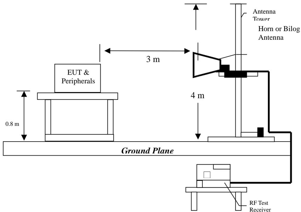
Radiated emissions were investigated cover the frequency range from 30MHz to 1000MHz using a receiver RBW of 120kHz record QP reading, and the frequency over 1GHz using a spectrum analyzer RBW of 1MHz and 10Hz VBW record Average reading. (15.209 paragraph), the Peak reading (1MHz RBW/VBW) recorded also on the report.
