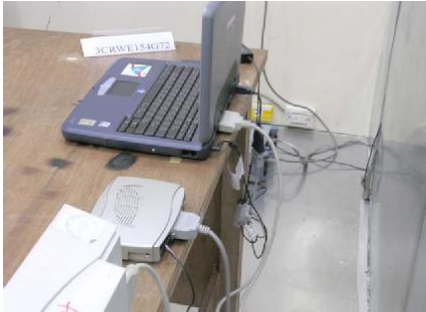
Photo 2: Conducted Test Set-up (rear)
