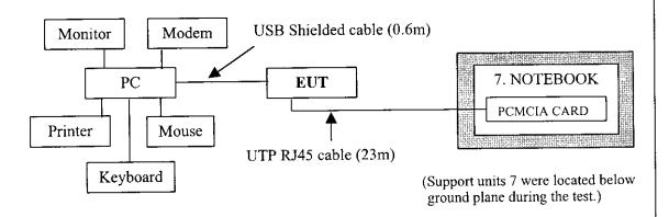
Both conducted and radiated testing were performed according to the procedures in ANSI C63.4:1992. Radiated testing was performed at an antenna to EUT distance of 10 m on an open area test site. Please refer to the photos of test configuration in Item 5.
