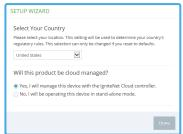
Select the country of operation for the AP. Setting the correct country ensures that the radios operate within local regulations specified for Wi-Fi networks.
