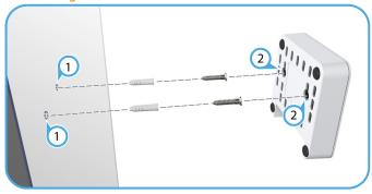
1 At the installation location on the wall, mark two holes 44 mm (1.73 in) apart for the wall plugs and screws (not included).
