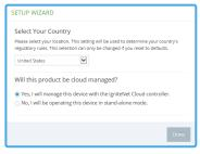
Select the country of operation for the AP. Setting the correct country ensures that the radios operate within local regulations specified for Wi-Fi networks.
