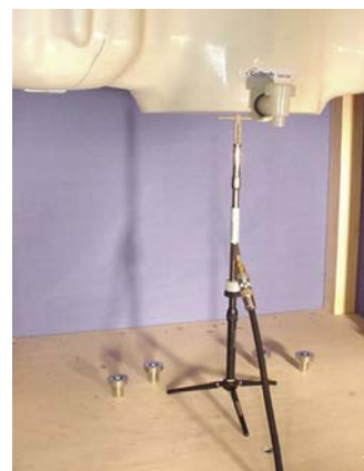
1800MHz Dipole Setup
