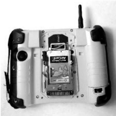
A software driver needs to be installed to activate the card.
