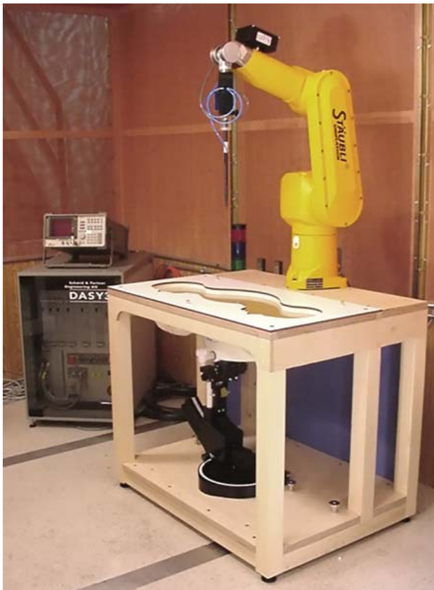
DASY3 SAR Measurement System with SAM phantom
