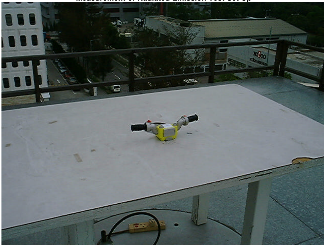
Measurement of Radiated Emission Test Set Up
