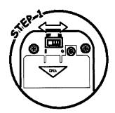
Turn on vehicle by sliding on-off switch on underside of chassis. Vehicle will start to spin
