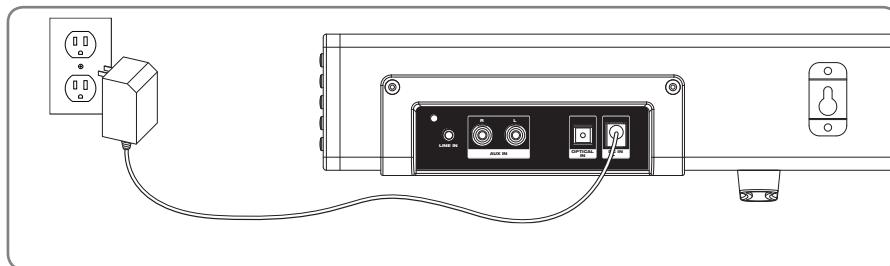
Plug the small end of the power cord into the DC Input on the back of the speaker, and the large plug into a standard wall outlet.
