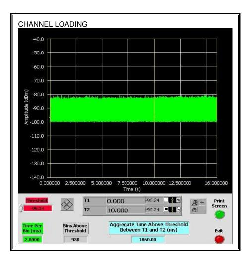
The level of traffic loading on the channel by the EUT is 18.6%
