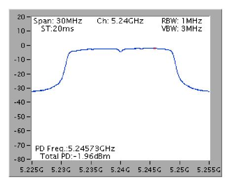
Power Density Plot on Configuration IEEE 802.11n MCS0 HT40MHz / / Ant. 1 + Ant. 2 + Ant. 3 / 5230 MHz
