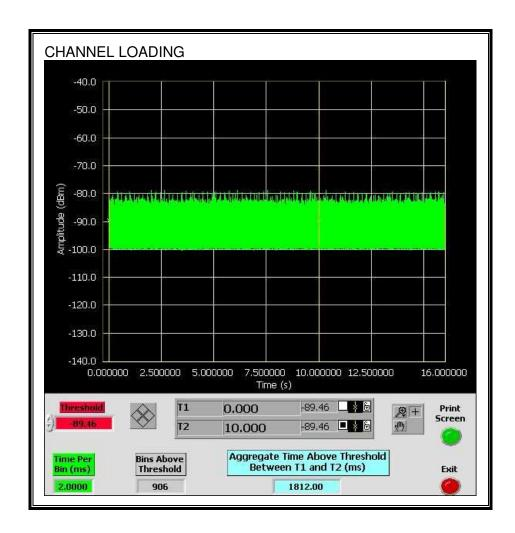
The level of traffic loading on the channel by the EUT is 18.12%
