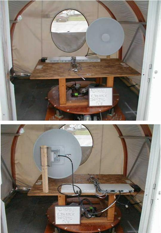
Radiated Emissions Test Setup Parabolic Antenna
