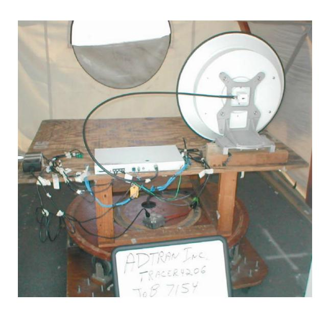
**Conducted Spurious Emissions Test Setup**
