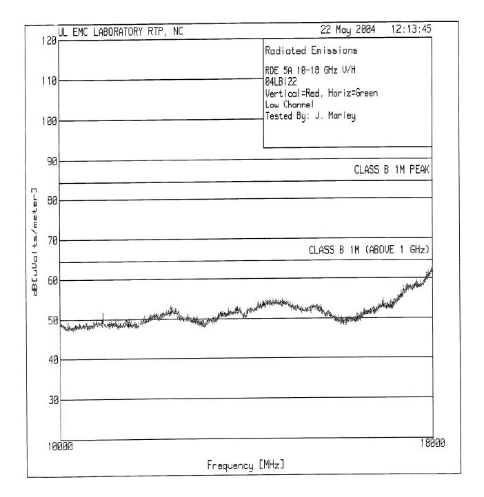
Test 5, Item B - Peak Plot, High Channel (Amplitude in dBuV/m):
