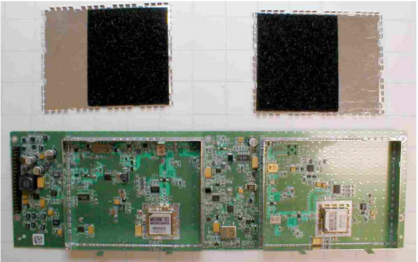
RF Board Bottom, Shields Removed
