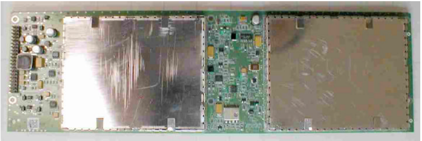
RF Board Bottom, Shields In Place
