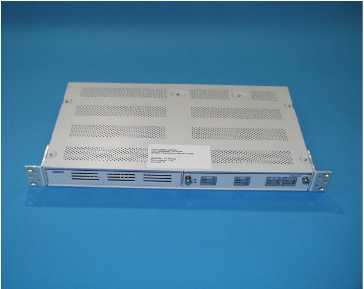
Photograph 4.14: Baseband Processor Assembly Front View
