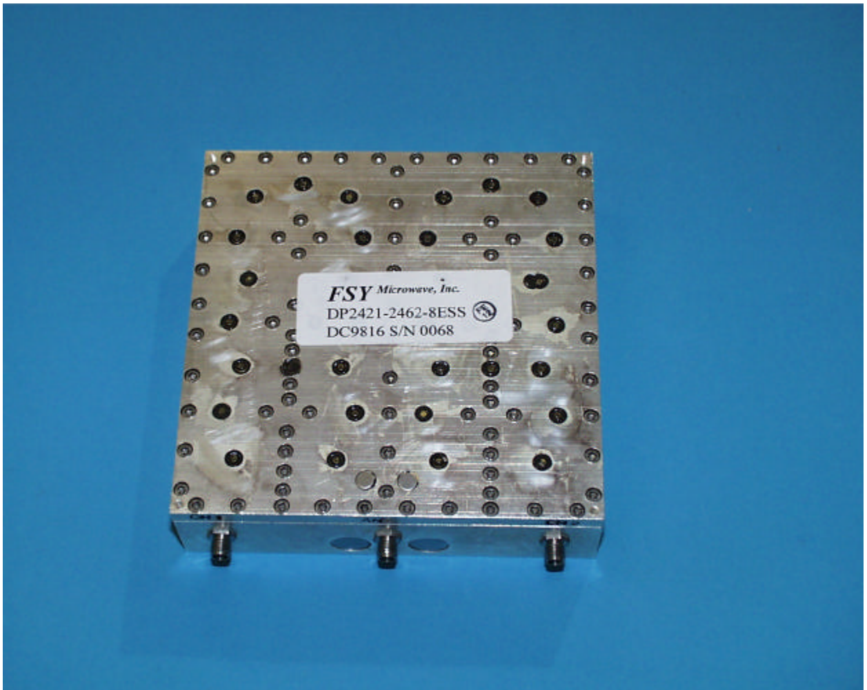
Photograph 4.12: Diplexer/Filter Top View
