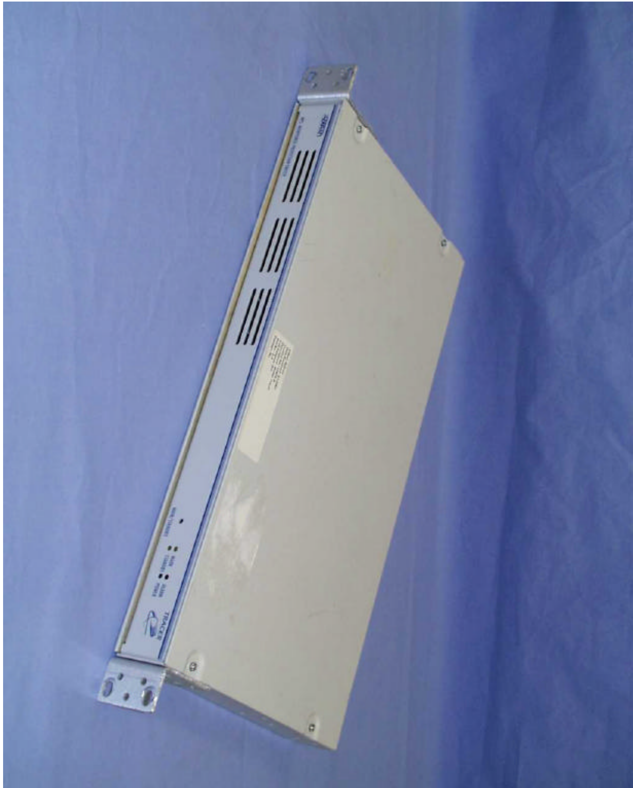
Photograph 2.1 Tracer Monitored Protection Switch Front / Top View
