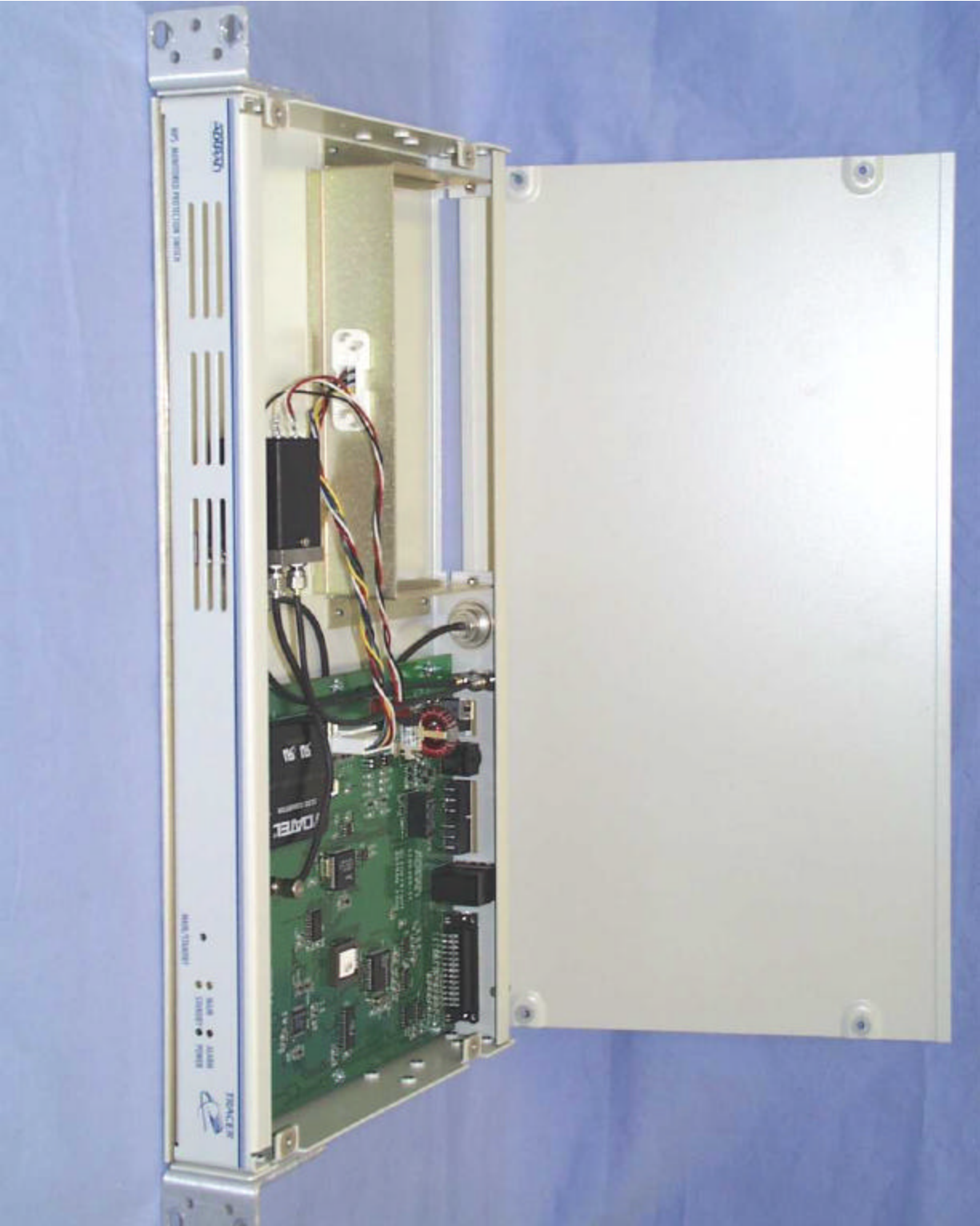
Photograph 2.5 Tracer Monitored Protection Switch Inside Chassis
