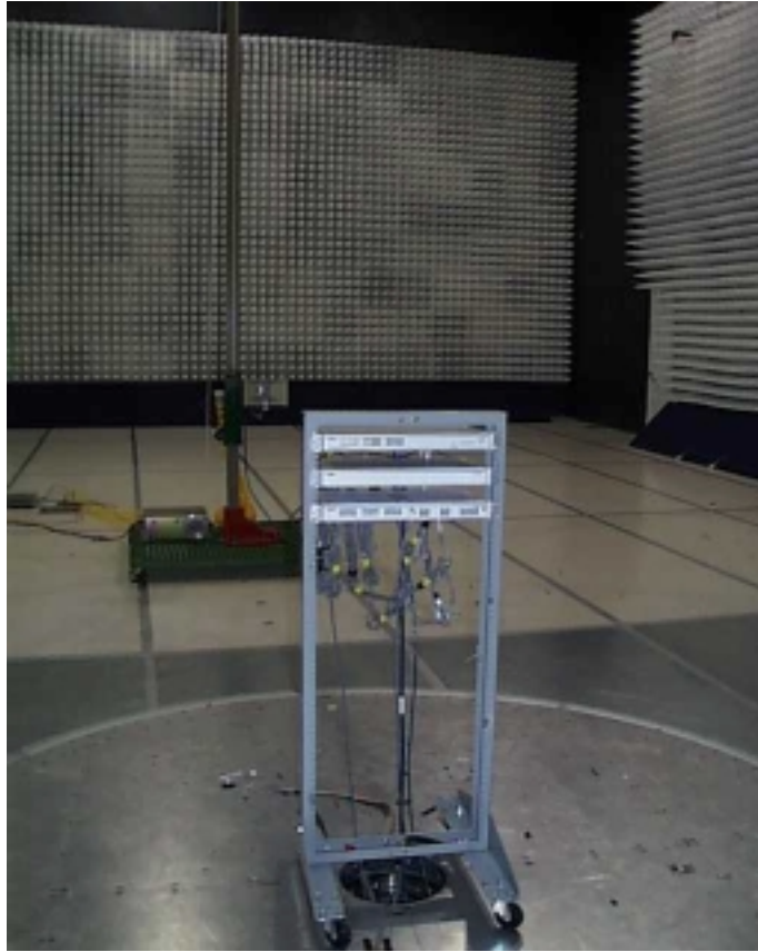
Figure 7: Worst Case Radiated Emissions Setup – Front View
