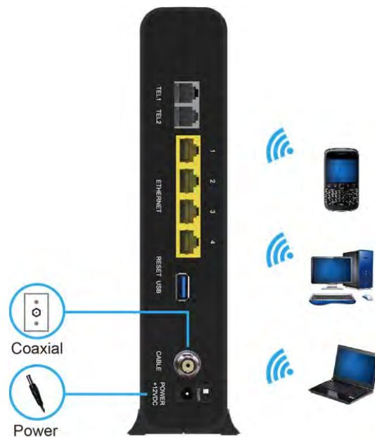
Sample Wireless Network Connections (SR820ac model shown)
