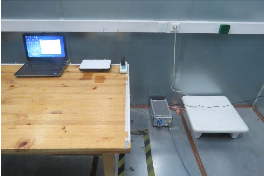
Picture 3 Conducted Emission Test Setup
