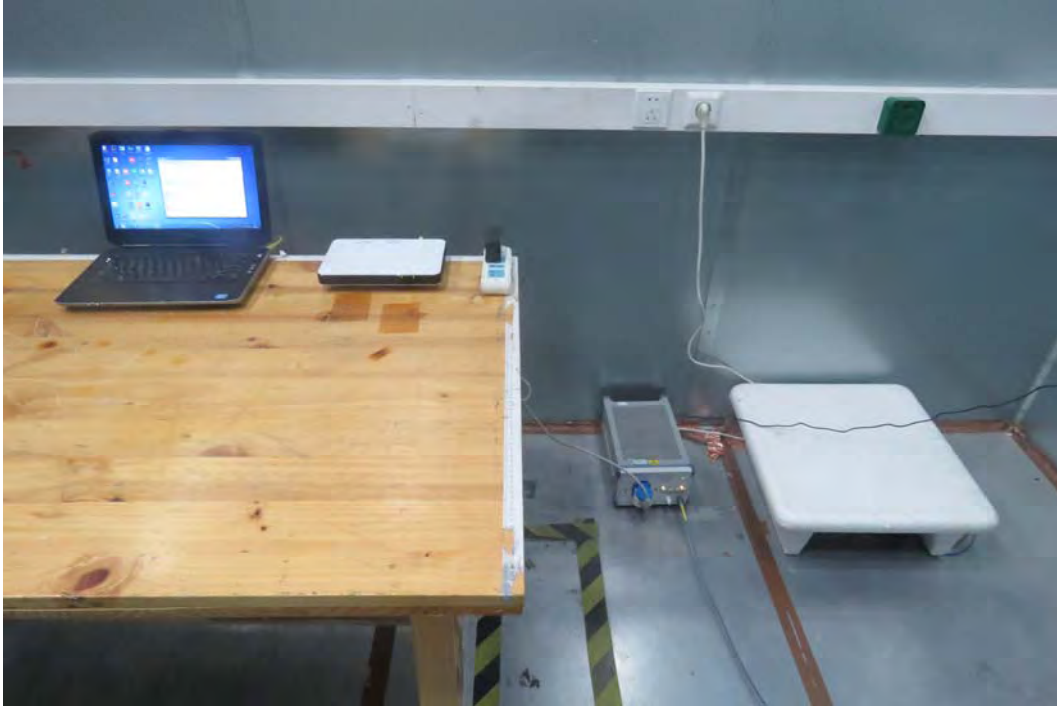
Picture 3 Conducted Emission Test Setup
