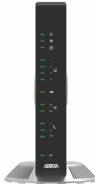
Figure 2. 434RG ONT with Base Attached
