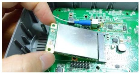
Step3: Assemble with necessary screws. 2pcs per unit.
