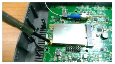
Step4: Assemble the antenna, 2pcs per unit
