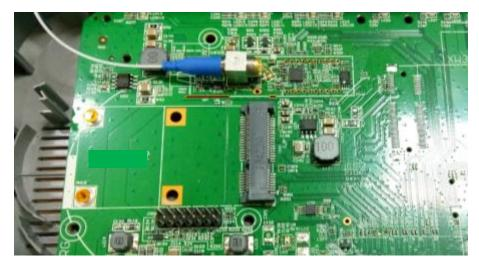
Step2: Assemble XW325EG in the miniPCle socket.
