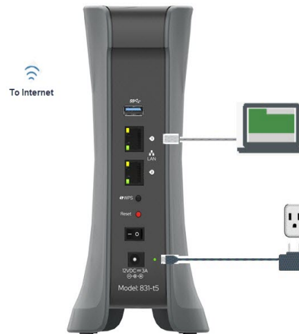
Figure 2. 831-t5 Gateway Installation Options (placeholder)
