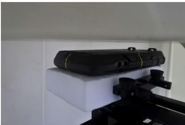
Rear Face, Test Separation 10 mm
