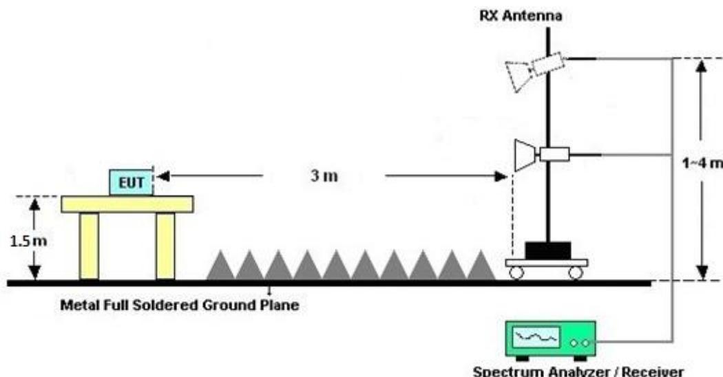
For radiated test above 18GHz
