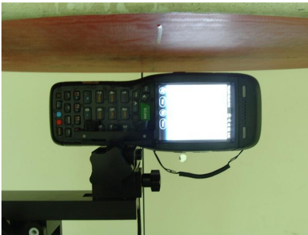
Left side of the DUT with Phantom 1.5 cm Gap
