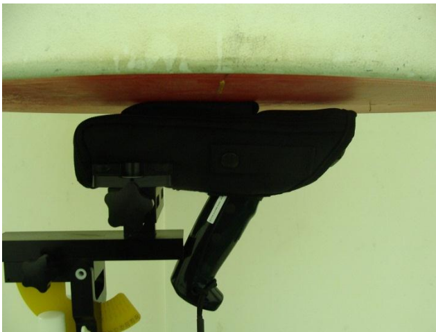
Front of the DUT with Holster with Phantom 0 cm Gap
