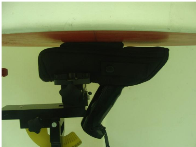
Front of the DUT with Holster with Phantom 0 cm Gap
