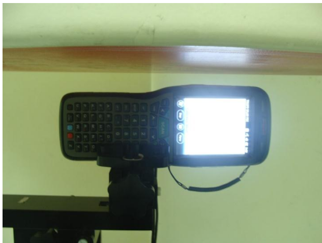
Left side of the DUT with Phantom 1.5 cm Gap
