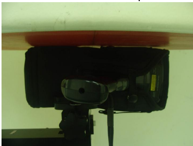
Right side of the DUT with Holster with Phantom 0 cm Gap
