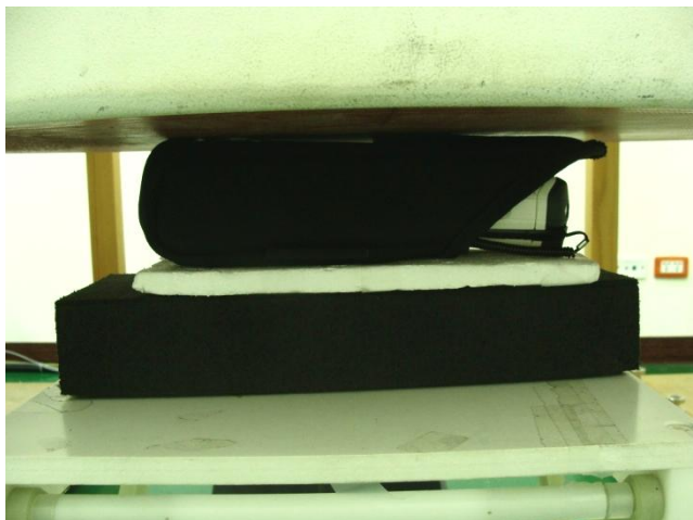
Face of the DUT with Holster with Phantom 0 cm Gap
