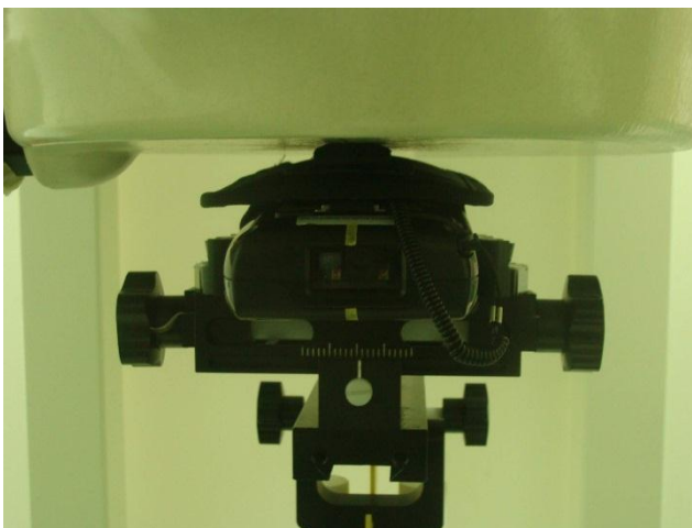
Back of the DUT and Holster with Phantom 0 cm Gap
