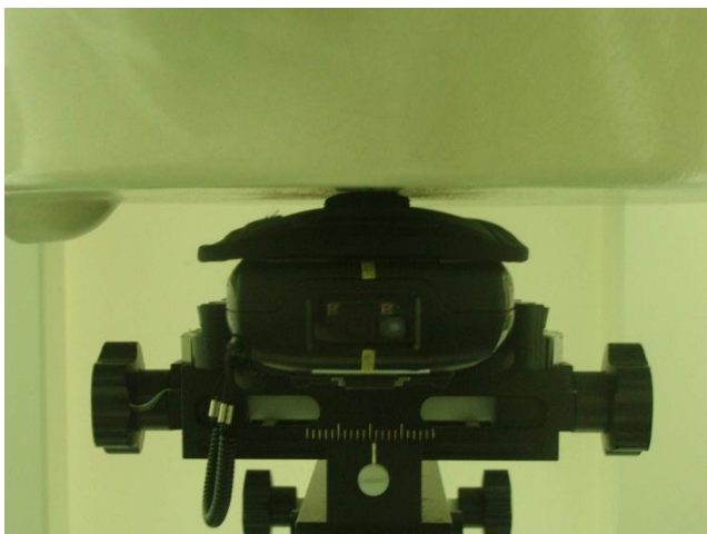
Front of the DUT and Holster with Phantom 0 cm Gap
