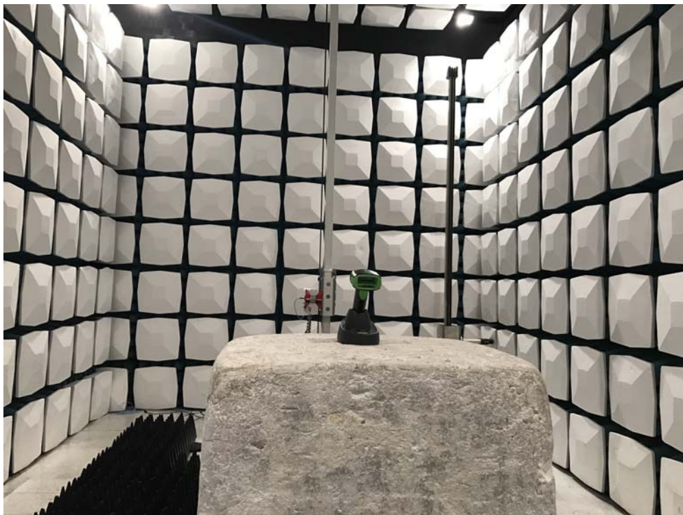
Description: Radiated Emission Test Setup for 1~18GHz
